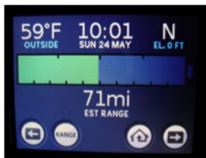
Sample of battery ½ depleted.
