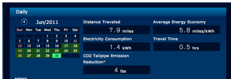
The sedan has a web portal for energy use by car, daily etc. But readouts for miles/kWh appear inflated, even if data are battery to motor only.
